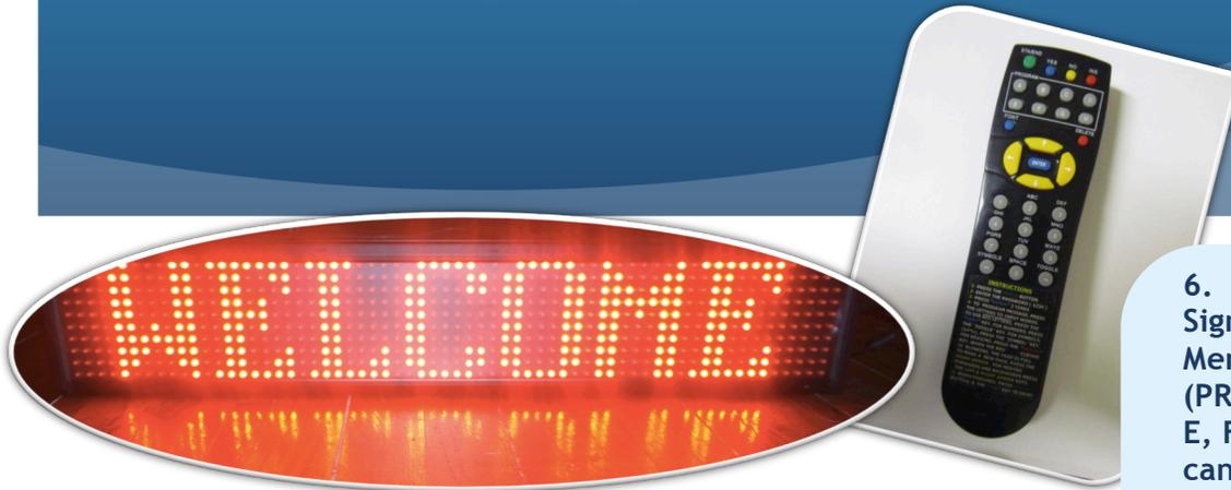
1. Press the GREEN “STA/END” button on the top left of the remote to stop the sign, Enter the UNIQUE 4 DIGIT PASSWORD ,then Press the BLUE “ENTER” button 2 times.
