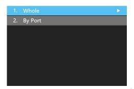
In the sub-menu, you can select **Whole** or **By Port** to control the movement of the display on LED screen. In **Whole** interface, you can set the starting point (X, Y) of the entire display image; In **By Port** interface, you can set the starting point (X, Y) of the display image for each of the 16 ports respectively. You should save the settings when you finish.
