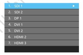
In the sub-menu, you can access the setting interface for any of the signals via the **Knob/OK** button. The setting items include: coordinates of the starting point (**X** and **Y**), **Width**, and **Height**. You should save the settings when you finish.
