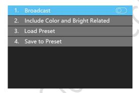
In the sub-menu, you can enable/disable **Broadcast**, and save up to 16 sets of preset, with each preset containing all parameters of the video source (scaling, cropping, multi-window display, EDID, etc.). In addition, you can also load and apply a saved preset, without the need to set the parameters one by one. Note that there are 4 sets of preset saved in the processor by default.
