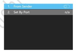
In the sub-menu, you can enable/disable **From Sender** (send the mapping parameters from sender to receiver). When **From Sender** is enabled, you can access the **Set By Port** interface to select the port (Port 1-16) for setting mapping. You can then set the offset value and determine the width, height, row count, and column count of the cabinets (tiles) controlled by the selected port. When you complete the settings, you should save the settings via the **Knob/OK** button.
