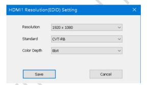
Click the downward arrow at the right side of **Resolution** field to bring up the drop-down menu of available resolution options. You can also customize the resolution by selecting **Custom** in the menu.
