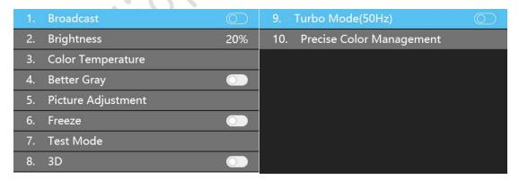
Broadcast: When Broadcast is selected, you can rotate the Knob/OK button to enable or disable it. With Broadcast enabled when there are multiple devices cascading, you can synchronize the adjustment made in one device to other devices.
