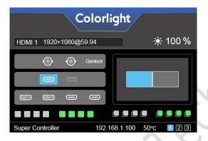
• **F2**: In any interface of the LCD in the front panel, you can press **F2** button to jump to the interface of signal list.
