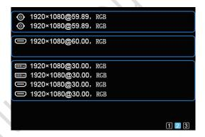
• **F3**: In any interface of the LCD in the front panel, you can press **F3** button to jump to the interface for switching signals.
