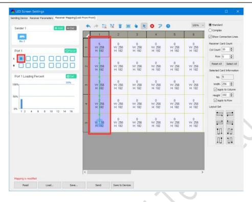
For a situation where cabinets of multiple specifications (different dimensions) exist, you can adjust the different cabinets independently after the settings.
